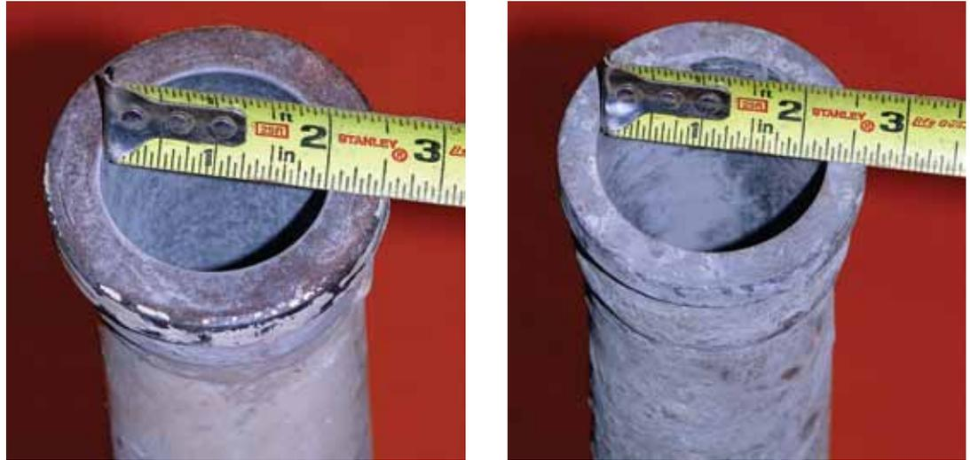
Fig. 1: Reducer A (left) is in new condition. Interior diameter is 2 in. (50 mm). Reducer B (right) displays obvious wear. Interior diameter is 2-1/4 in. (56 mm)
