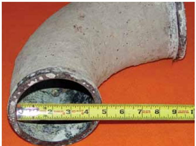
Fig. 3: Elbow A (left) displays a 4 in. (101 mm) interior diameter. Elbow B (right) measures 4-5/16 in. (109 mm)
