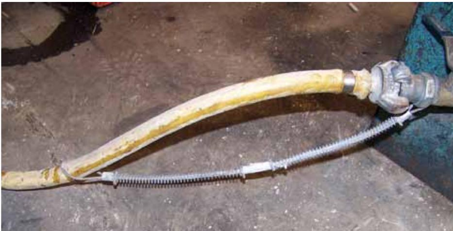
*Use of whip checks with pneumatic tools at each connection point*
