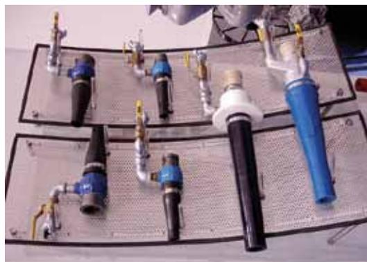
Fig 1: A few of the countless wet-mix nozzles currently available
