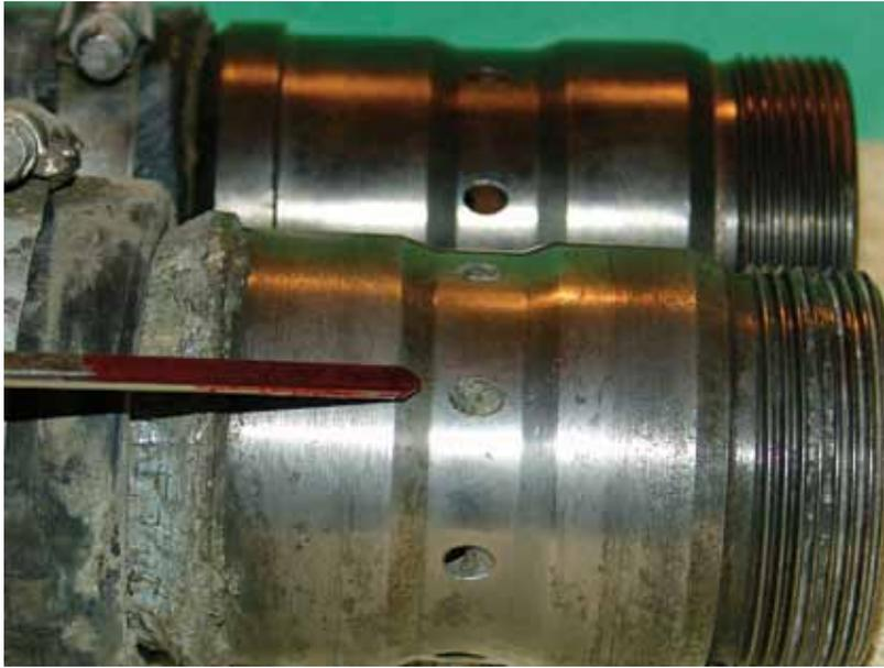
Fig 4: Note plugged port within nozzle body
