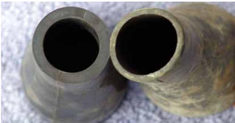
Fig 6: After placing only 80 lb/yd<sup>3</sup> (60 kg/m<sup>3</sup>), the worn tip on the right has become oversized and must be discarded
