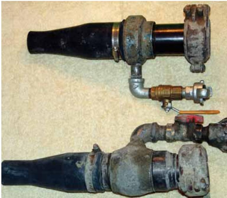
Fig 7: Note undersized 1/2 in. (13 mm) elbow and valve on upper nozzle and properly sized 3/4 in. (19 mm) parts on nozzle below. Half-inch (13 mm) elbow and valve will not flow sufficient air for adequate shotcrete placement
