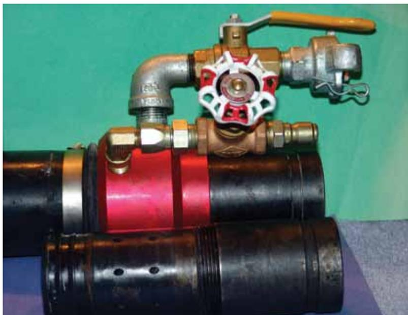
*Fig 2: Note second valve supplying second row of drilled ports on wet-mix admixture nozzle*
