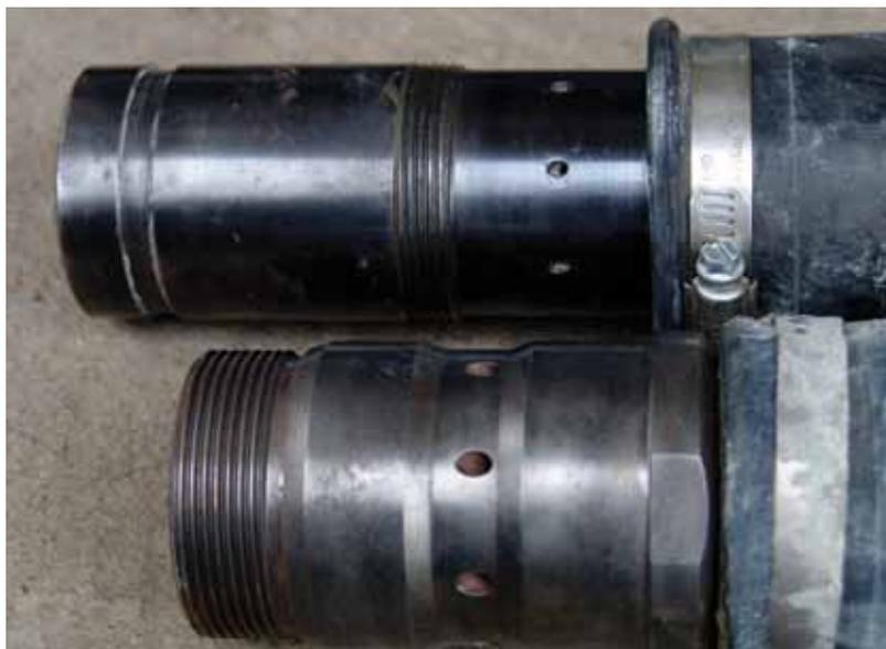
*Fig 3: Nozzle body above with 1/8 in. (3.2 mm) drilled ports. Nozzle body below uses 3/16 in. (5 mm) ports and adds chamfer to increase air flow*
