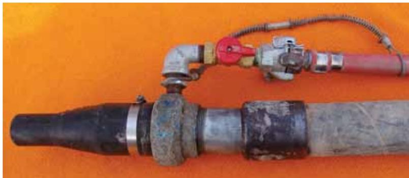
Fig 3: Two inch (50 mm) pipe thread acts as nozzle coupler
