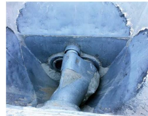
Fig. 2: A wet-mix pump with missing auger cannot effectively fill material cylinders. Unpredictable flow and slugging will affect nozzleman placement quality
