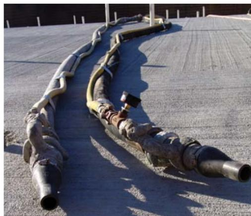
Fig. 1: Although visibly similar, nozzle end hoses may feel very different to a nozzleman. Choose an end hose that is sufficiently rigid, not “doughy”
