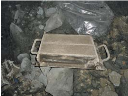
Fig. 3: End beams in a steel mold after shooting underground
