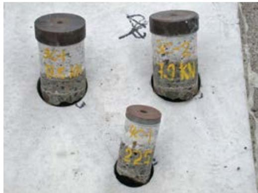
Fig. 5: Extracted cores after pulloff tests (photo courtesy of the CRIB)
