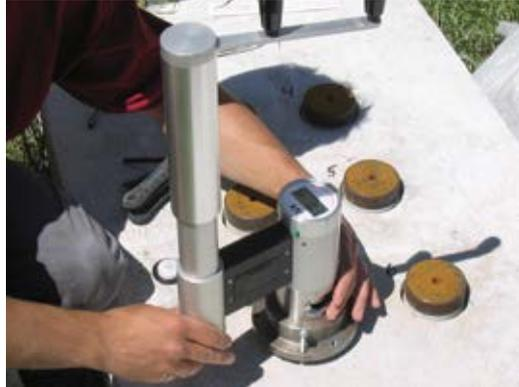
Fig. 4: A pulloff test being conducted on a test panel (photo courtesy of the Centre de recherche sur les infrastructures en béton (CRIB))
