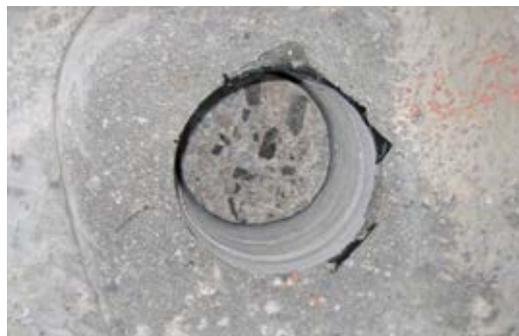
Fig. 6: A hole after a core has been extracted during a pulloff test
