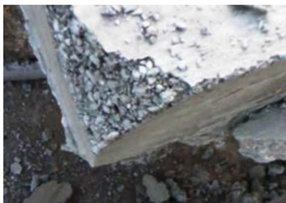
*Fig. 1: Poor placement techniques have produced sand lenses or encased rebound trapped within test specimen*
