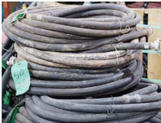
Fig. 7: Air supply line diameter is critical to maintaining adequate nozzle velocity
