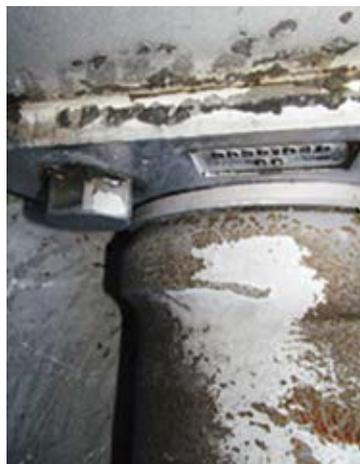
*Fig. 3(b): Wear components in good condition*
