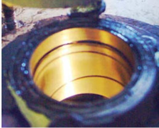
*Fig. 3: Properly lubricated shaft bearing at 3000 hours*
