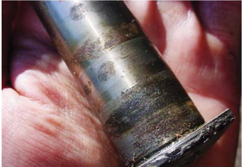
*Fig. 1: Unnecessary corrosion and wear on critical bearing surface is likely caused by improper grease application*
