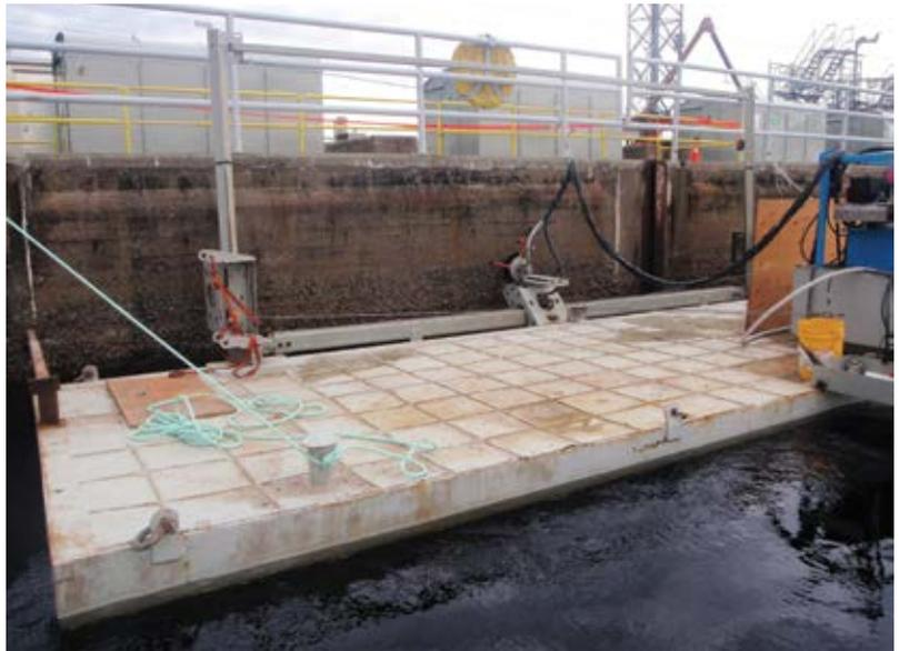
Fig. 2: Mobile hydrodemolition rig
