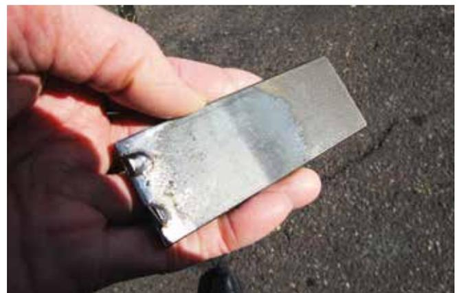
Fig. 3: Same metal plate after being halfway submerged in a high-alkaline (high-pH) water for 24 hours showing the formation of an iron oxide passivation layer (grayish-black)
