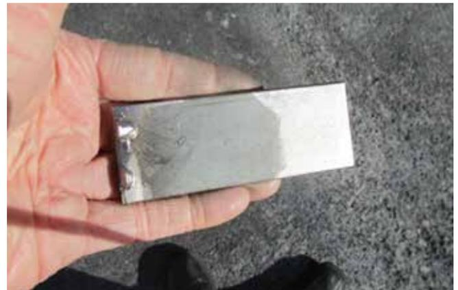
Fig. 2: Metal plate having one end that was ground down (shiny section) to expose virgin steel
