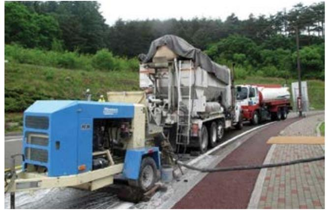
Fig. 3: Shotcrete pump with a mobile volumetric mixer
