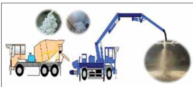
Fig. 2: Concept of cellular sprayed concrete
