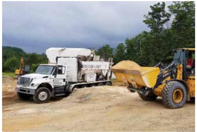
Fig. 1: Volumetric mixer truck on a pool shoot
